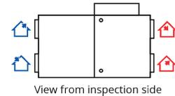
Exhaust air Extract air Outdoor air Supply air
